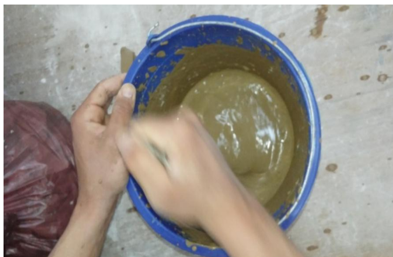
Figure III.13 : Barbotine d'argile pure.
