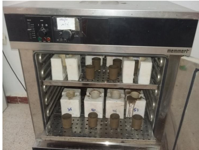
Figure III.19 : Séchage des biscuits.
